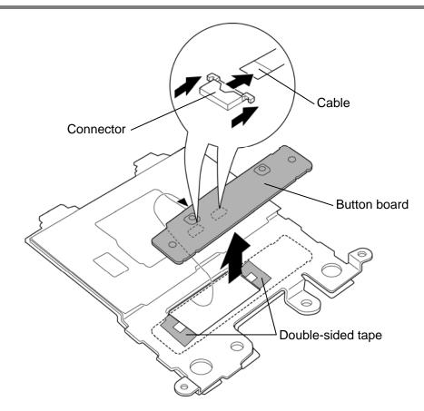
Figure 4-45 Removing the touch pad (2)
